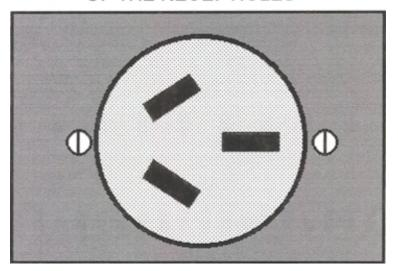
50 amp, Single Phase, 125/250 Volt, 3-Pole, 3-wire, (NEMA 10-50r receptacle) or 50 Amp, Single Phase, 125/250 Volt, 3-pole, 4-Wire Grounding (NEMA 14-50r receptacle). See diagram at left.
