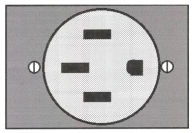
PROVIDE ONE OF THESE OUTLETS WITHIN 20 FEET OF THE STAGE.
